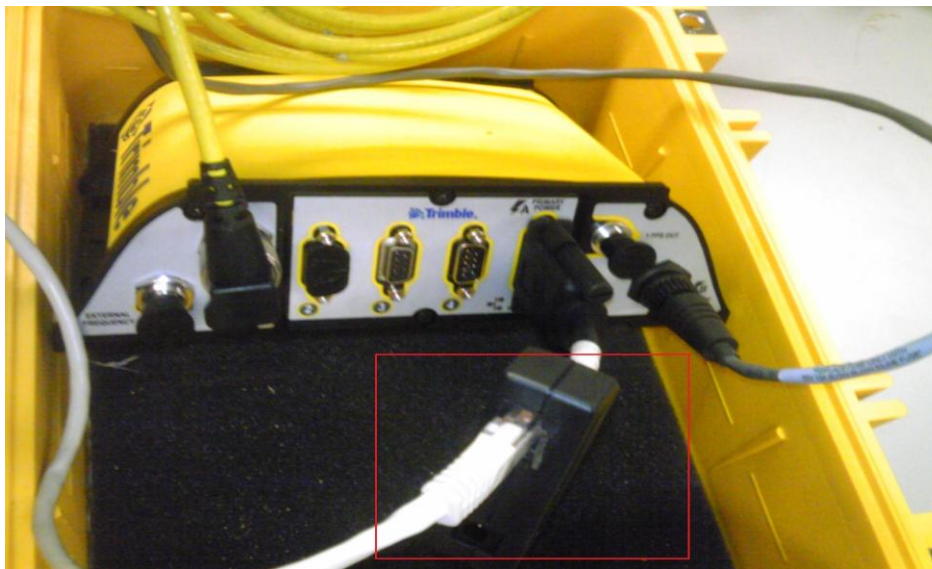
Figure A-1: Connection panel for Trimble receiver. Connection can be made through Ethernet cable (preferred) or serial cable
