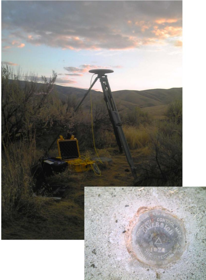
Figure 3: Photograph of NetRS and Trimble antenna data acquisition at the Diversion Benchmark (inset). NetRS receiver is housed in the yellow case and powered by a car battery
