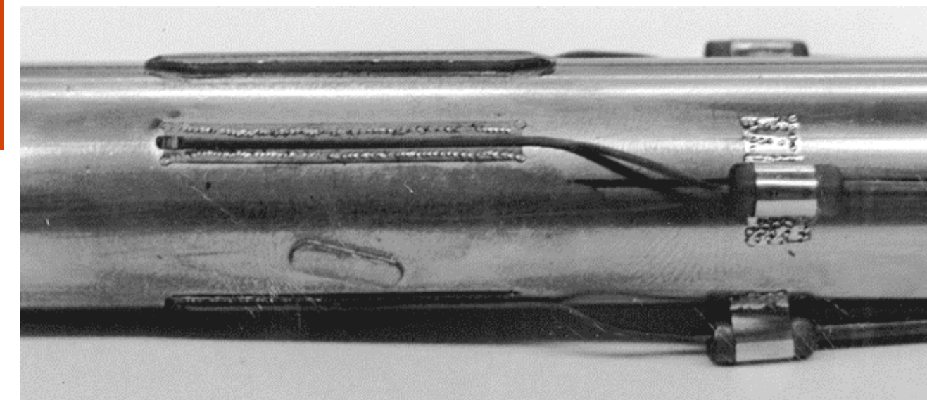
Figure 1: A strain gauge welded onto a nuclear fuel rod [2]
