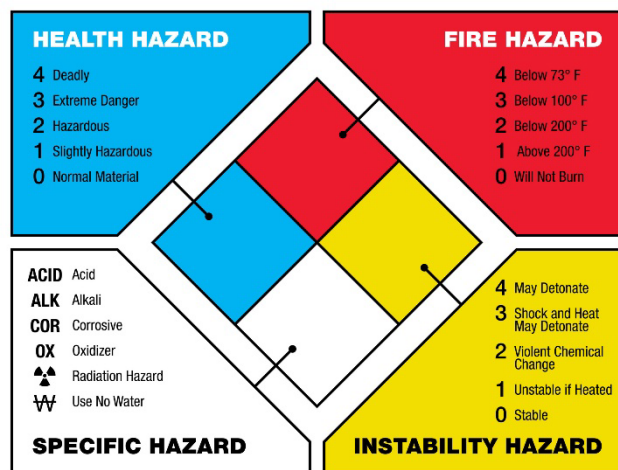
Figure 4.2 – Basic information detailed in an NFPA diamond and the HMIS signage
